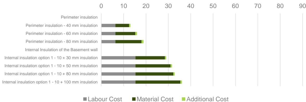
**Figure 5 - Component Cost France – Outer Walls Against Earth (Opaque Components)**
