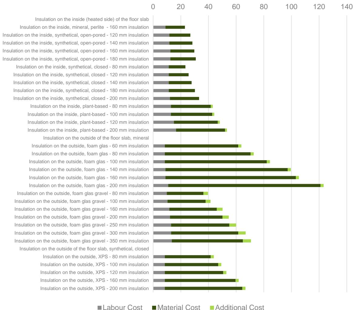
Figure 12 - Component Cost Germany – Basement (Opaque Components)
