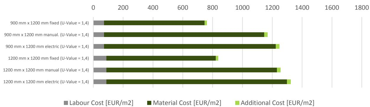
Figure 34 - Component Cost France – Windows in flat roof (windows)
