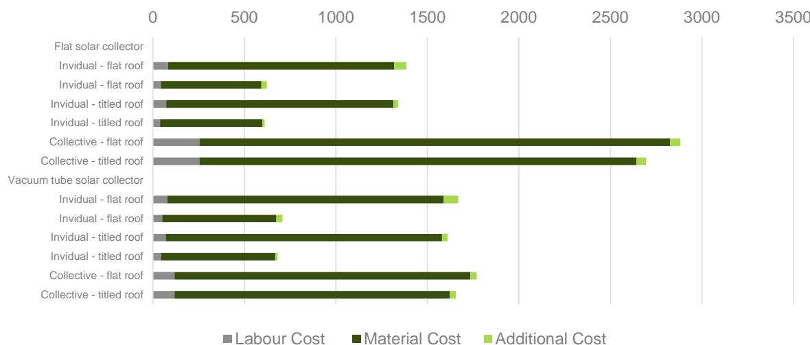
Figure 54 – Component Cost France – Solar Thermal
