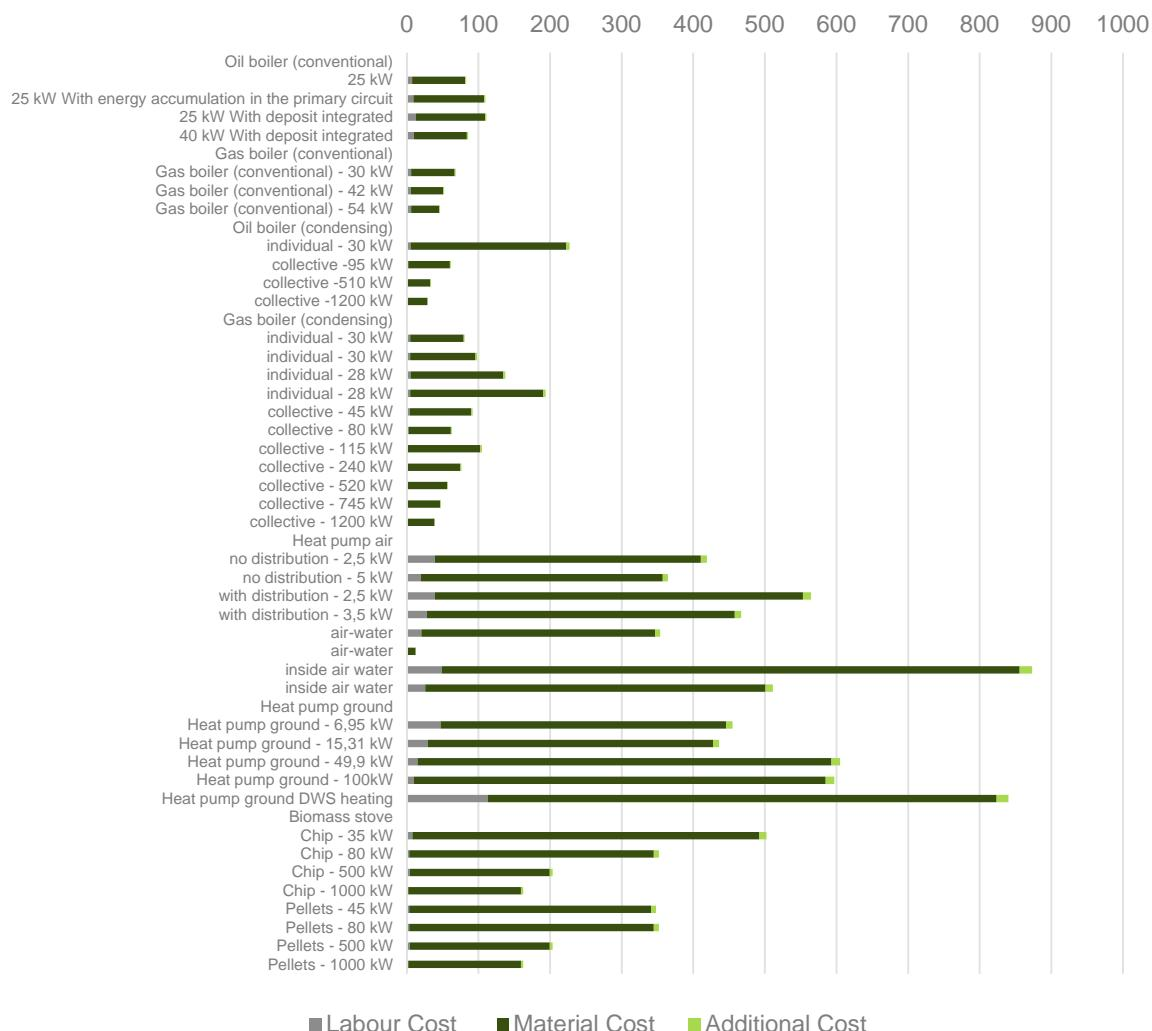
Figure 37 - Component Cost France (EUR/kWh) – Heating Systems
