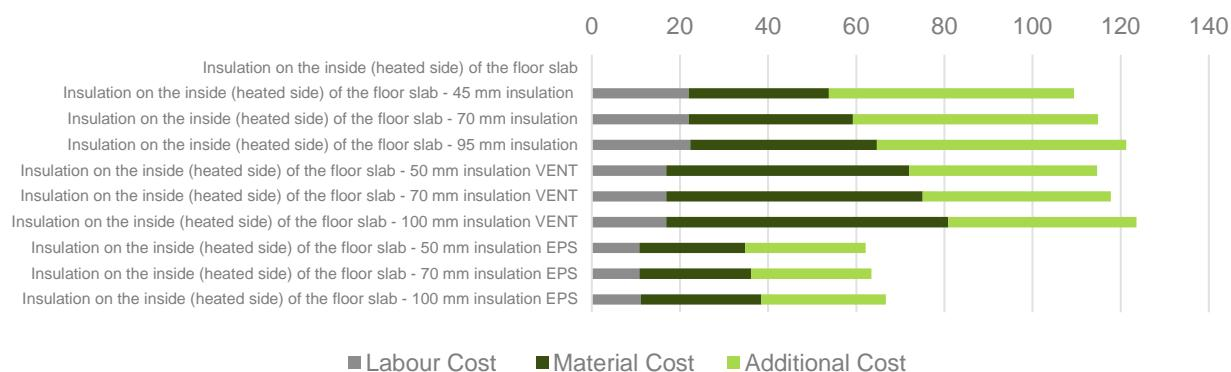
Figure 10 - Component Cost Sweden – Basement (Opaque Components)
