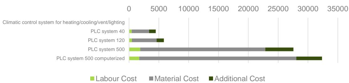
Figure 63 – Component Cost Sweden– Control Systems
