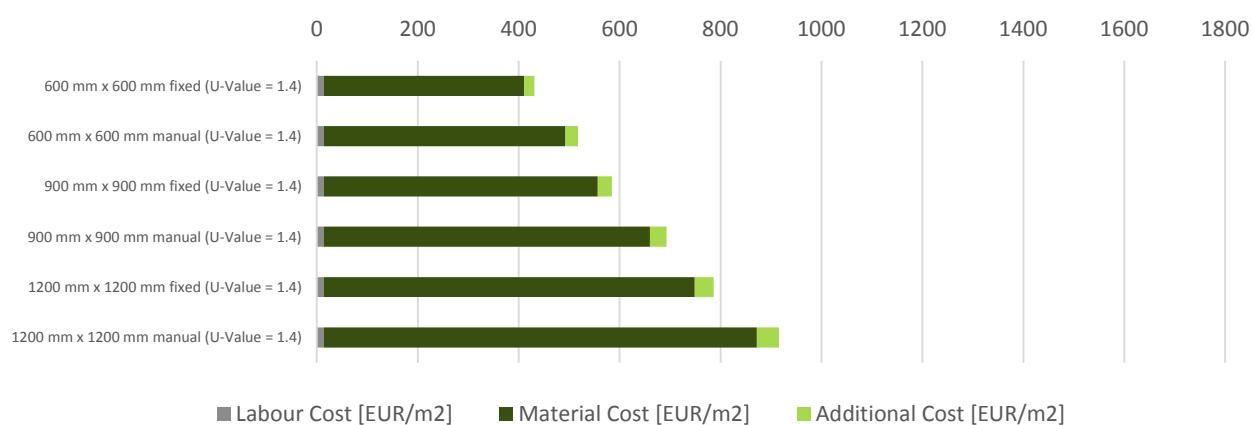
Figure 36 - Component Cost Spain – Windows in flat roof (windows)
