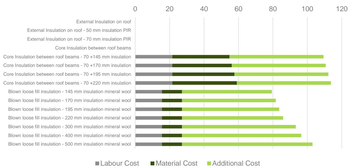
Figure 25 - Component Cost Sweden – Tilted Roof (Opaque Components)
