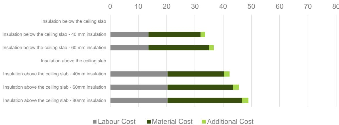
**Figure 18 - Component Cost Spain – Ceiling Against Unheated (Opaque Components)**
