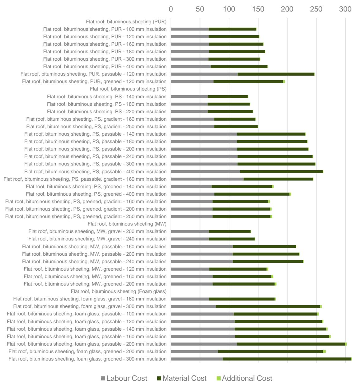
Figure 23 - Component Cost Germany – Flat Roof (Opaque Components)
