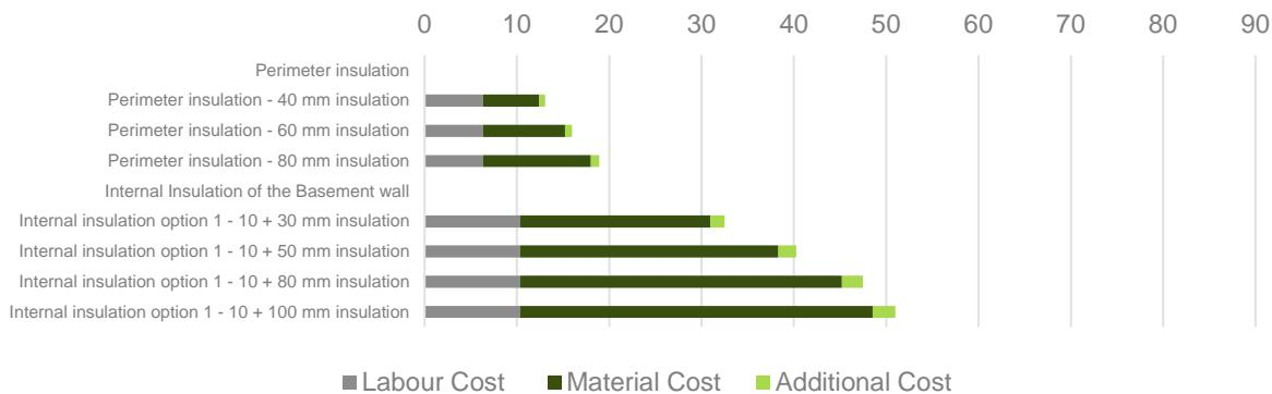
Figure 7 - Component Cost Spain – Outer Walls Against Earth (Opaque Components)
