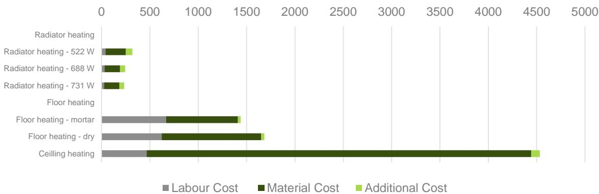
Figure 40 – Component Cost France – Heat Distribution
