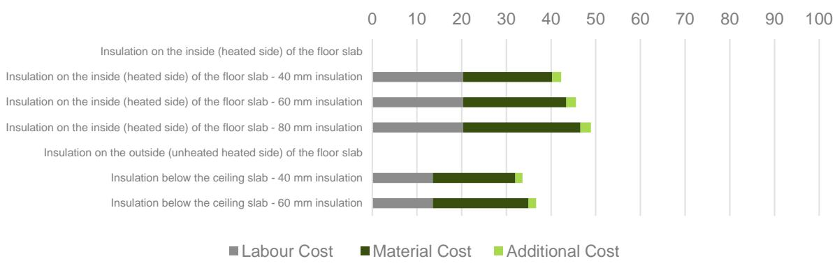
Figure 15 - Component Cost Spain – Floor Against Unheated (Opaque Components)
