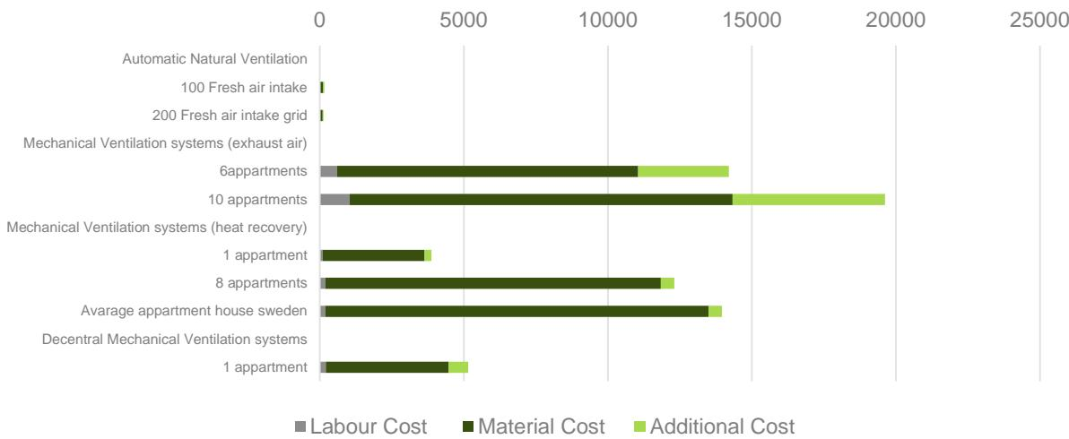
Figure 44 – Component Cost Sweden- Ventilation
