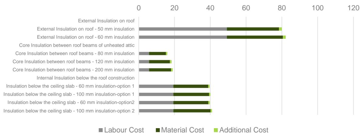
Figure 24 - Component Cost France – Tilted Roof (Opaque Components)
