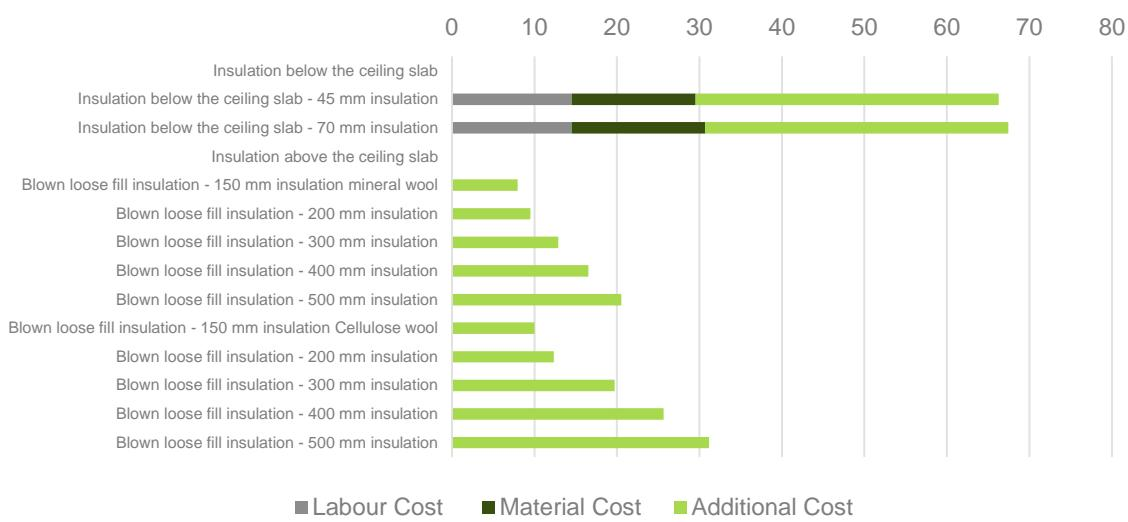
**Figure 17 - Component Cost Sweden – Ceiling Against Unheated (Opaque Components)**
