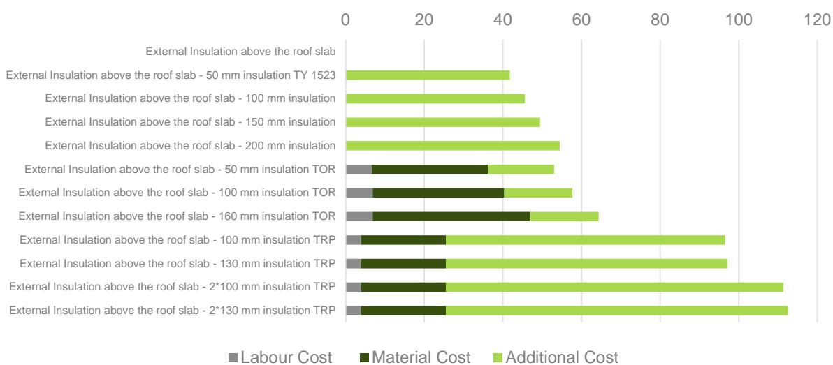
Figure 21 - Component Cost Sweden – Flat Roof (Opaque Components)
