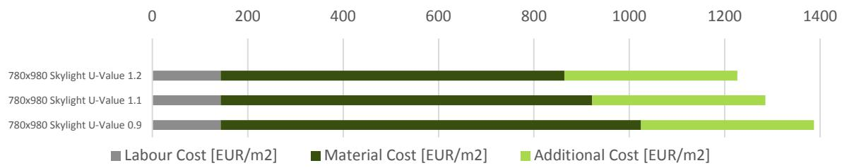
Figure 32 - Component Cost Sweden – Windows in tilted roof (windows)
