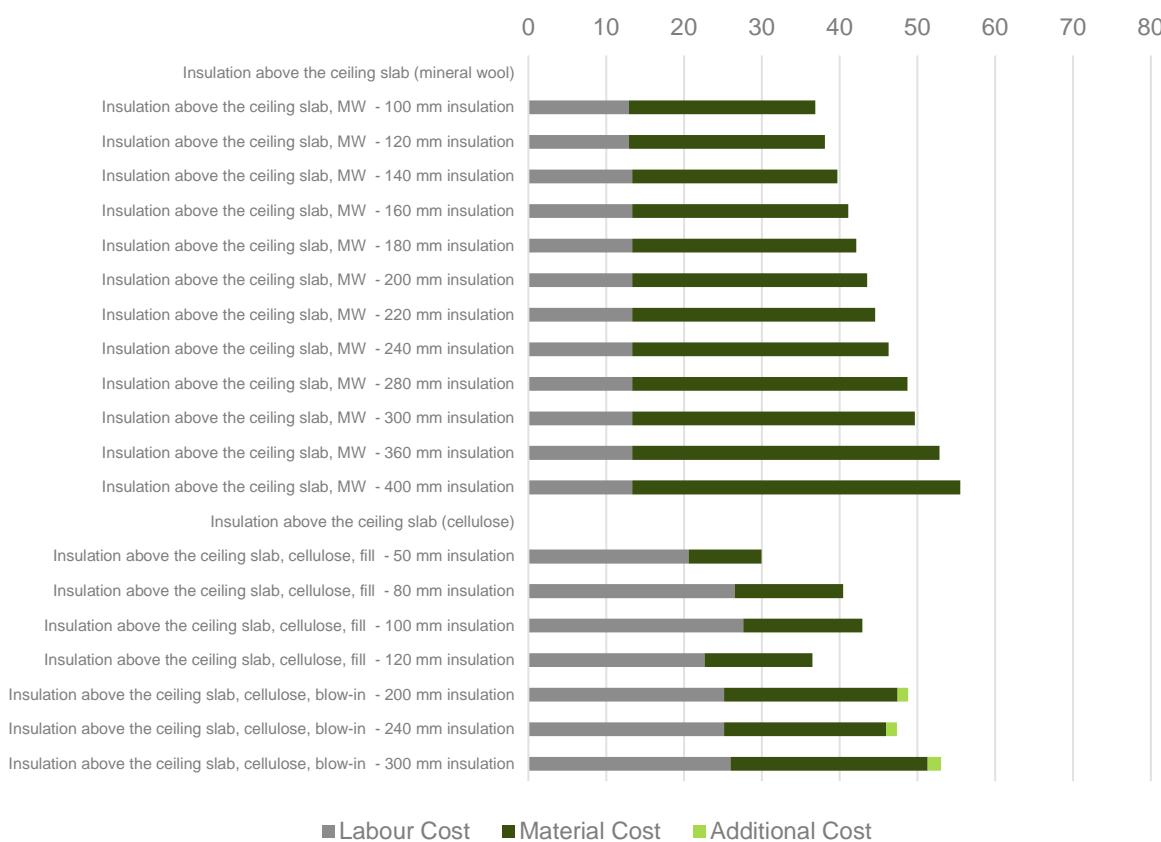
**Figure 19 - Component Cost Germany – Ceiling Against Unheated (Opaque Components)**
