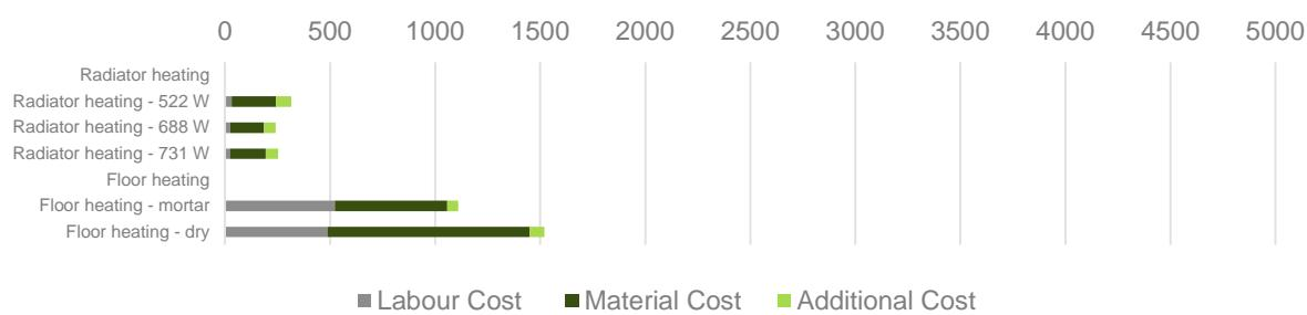
Figure 42 – Component Cost Spain – Heat Distribution
