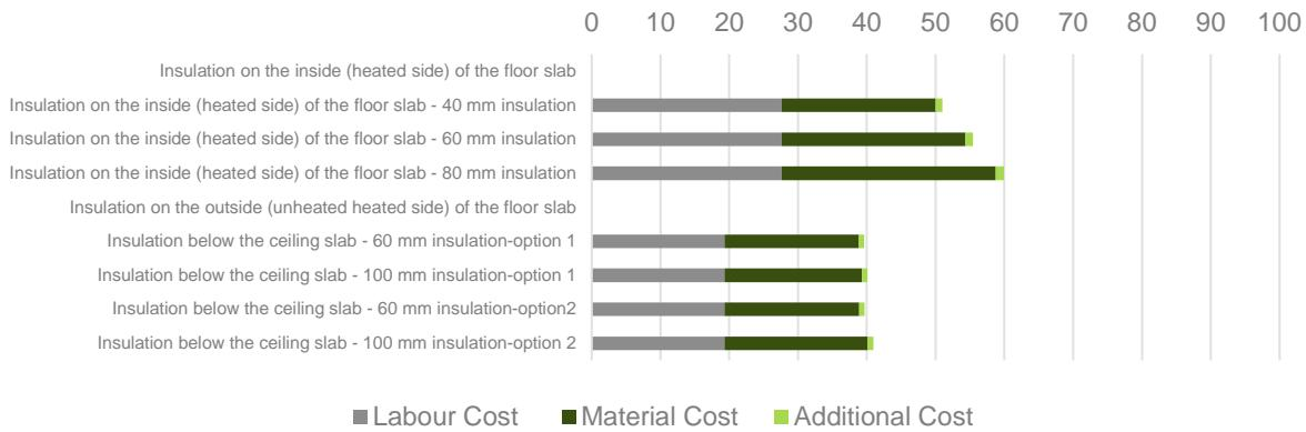
Figure 13 - Component Cost France – Floor Against Unheated (Opaque Components)
