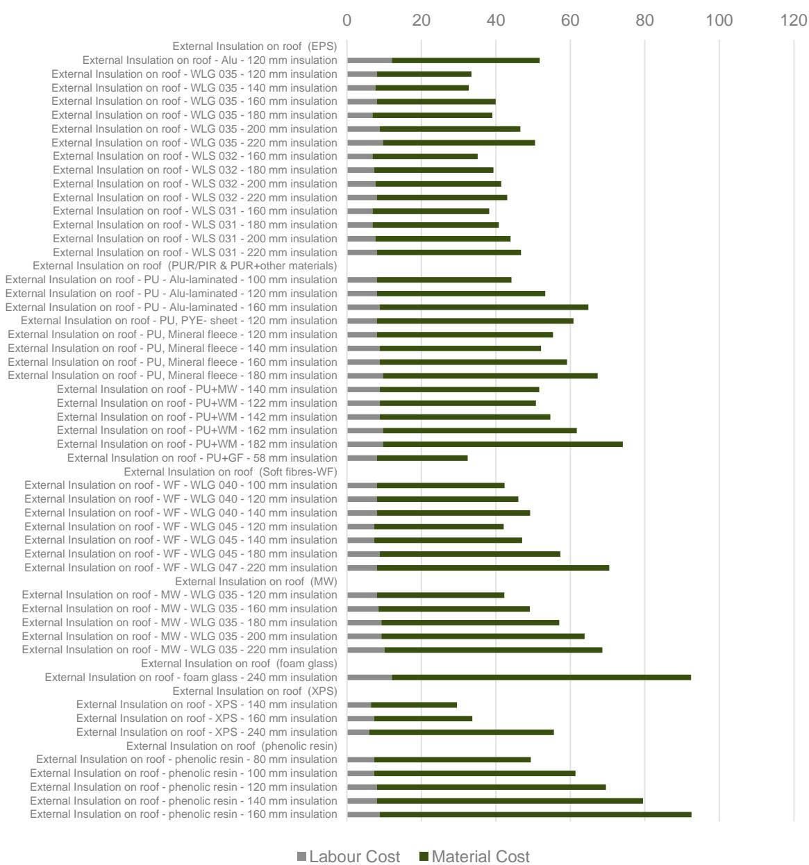
Figure 27 - Component Cost Spain – Tilted Roof (Opaque Components)
