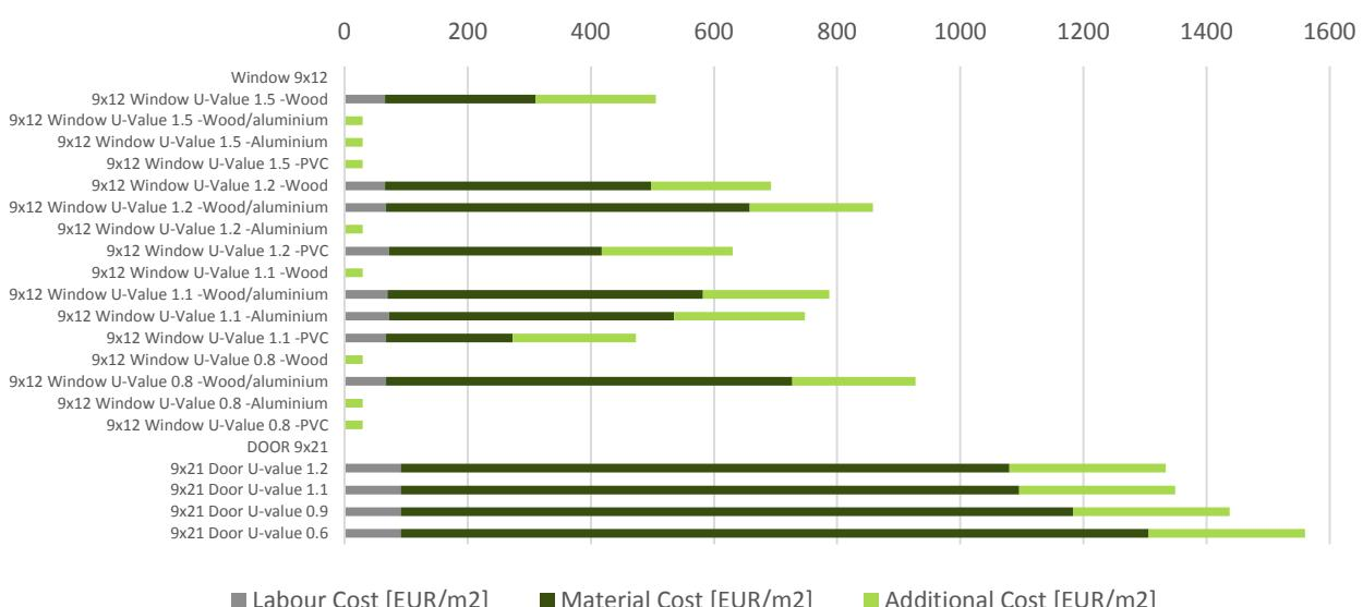
Figure 29 - Component Cost Sweden – Windows in wall (windows)
