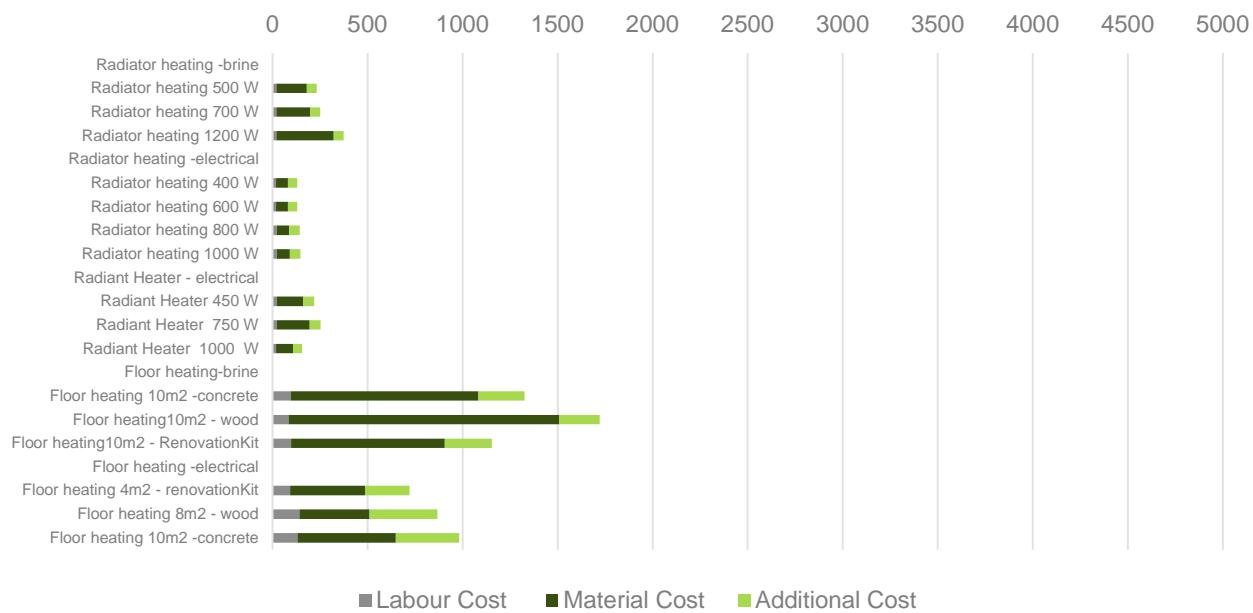
Figure 41 – Component Cost Sweden – Heat Distribution
