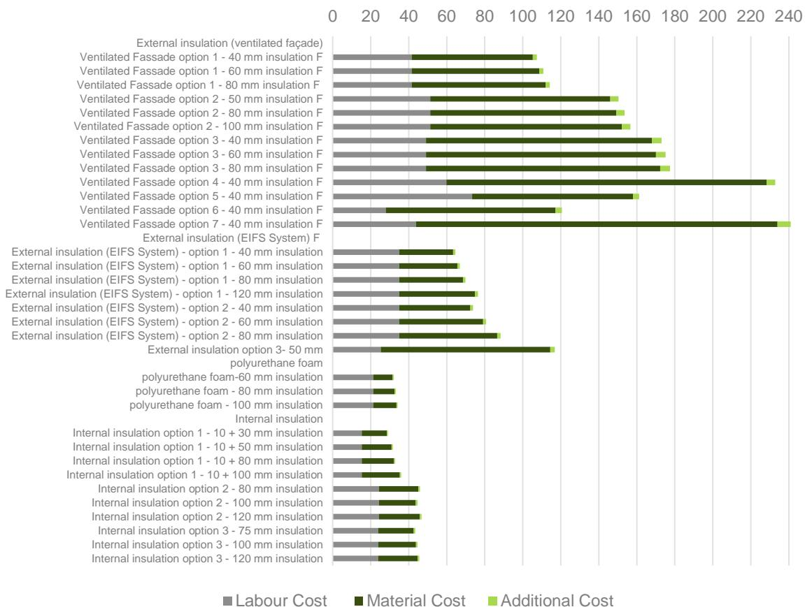
Figure 2- Component Cost France – Outer Walls Against Air (Opaque Components)
