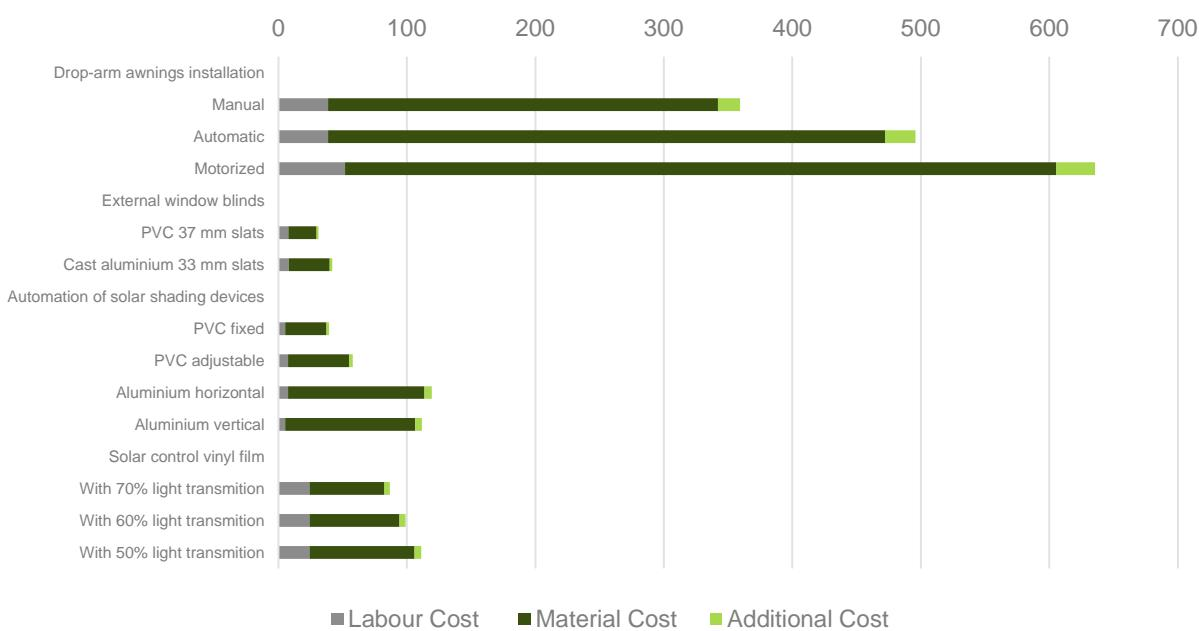
Figure 53 – Component Cost Spain – Shading
