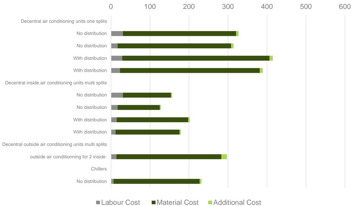
Figure 46 – Component Cost France – Cooling
