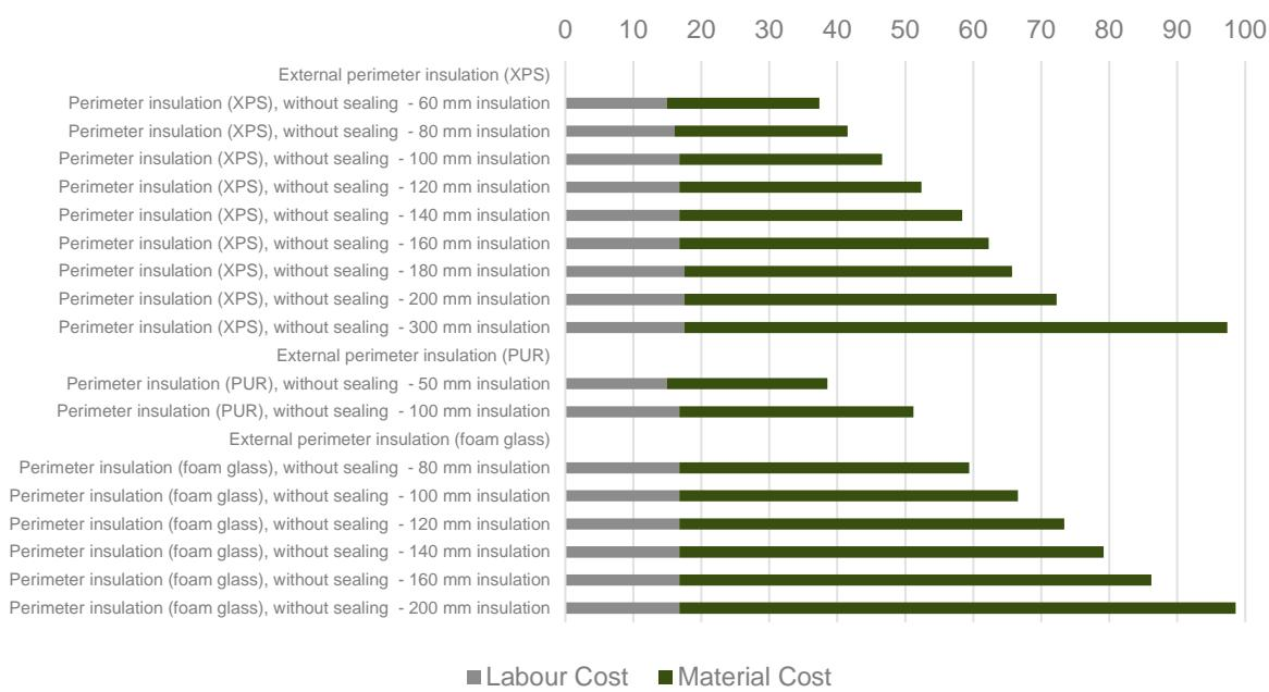
Figure 8 - Component Cost Germany – Outer Walls Against Earth (Opaque Components)
