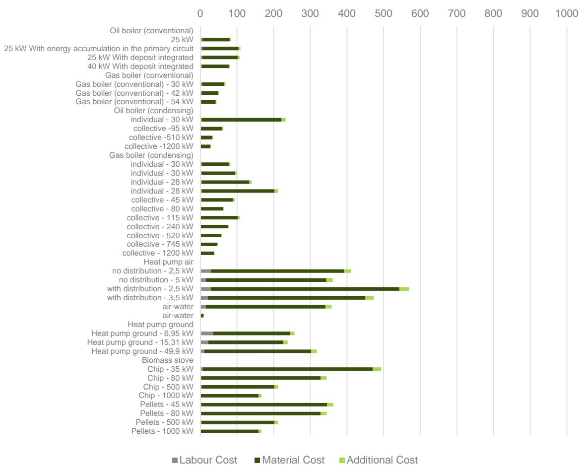
Figure 39 - Component Cost Spain – Heating Systems
