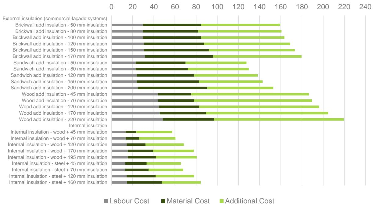
Figure 3 - Component Cost Sweden – Outer Walls Against Air (Opaque Components)
