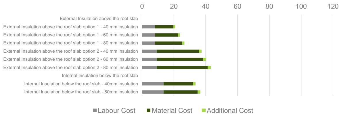
Figure 22 - Component Cost Spain – Flat Roof (Opaque Components)
