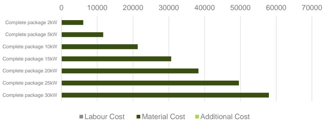
Figure 60 – Component Cost Sweden – Photovoltaic
