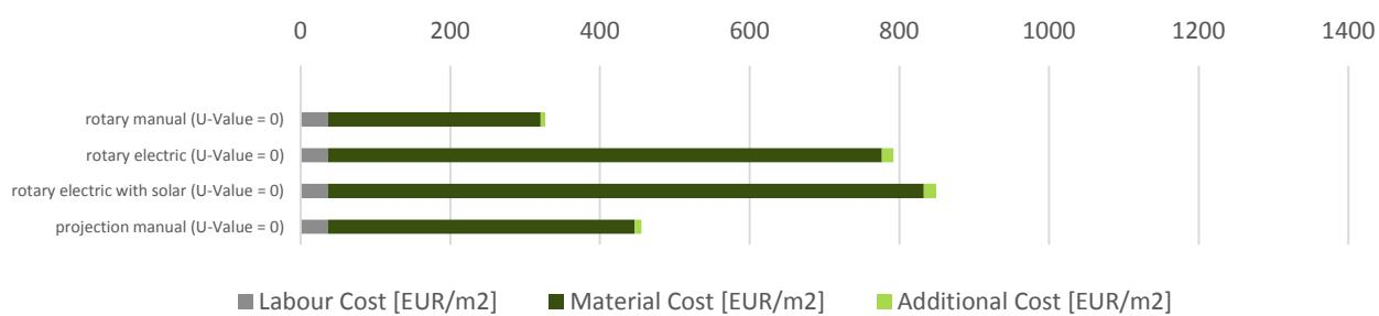
Figure 31 - Component Cost France – Windows in tilted roof (windows)
