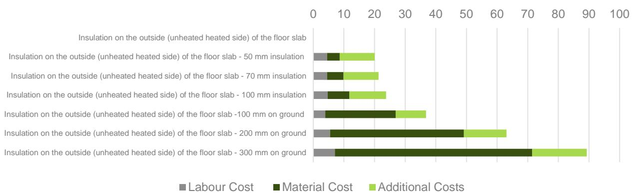
Figure 14 - Component Cost Sweden – Floor Against Unheated (Opaque Components)
