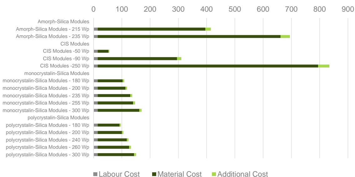
Figure 61 – Component Cost Spain – Photovoltaic
