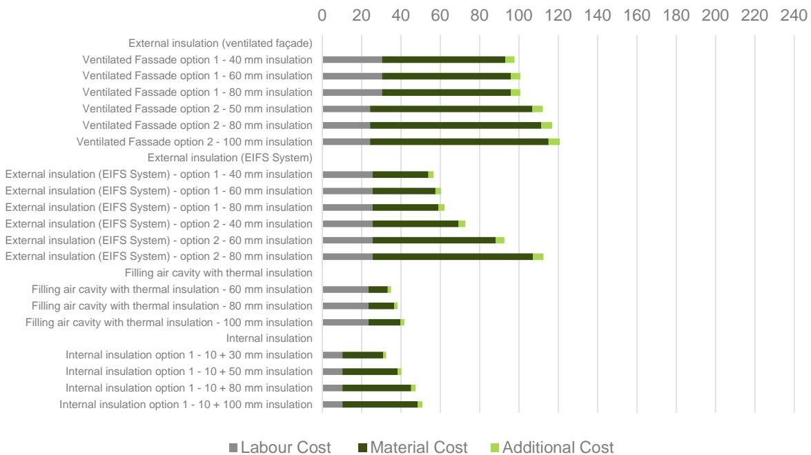
Figure 1 - Component Cost Spain – Outer Walls Against Air (Opaque Components)
