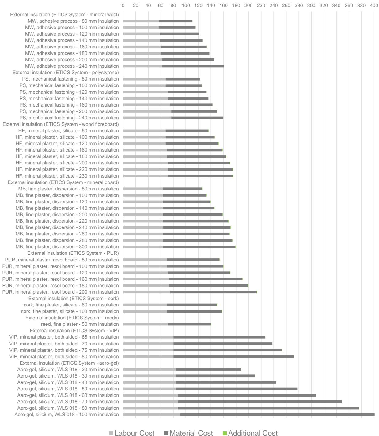
Figure 4 - Component Cost Germany – Outer Walls Against Air (Opaque Components)
