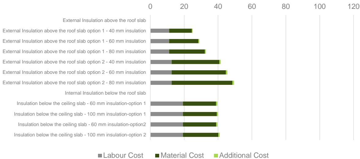
Figure 20 - Component Cost France – Flat Roof (Opaque Components)
