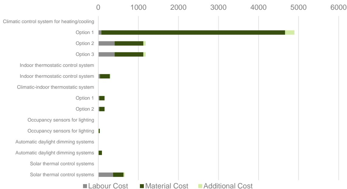
Figure 64 – Component Cost Spain– Control Systems
