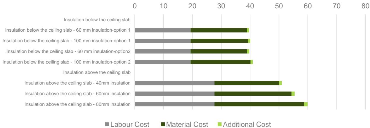
**Figure 16 - Component Cost France – Ceiling Against Unheated (Opaque Components)**
