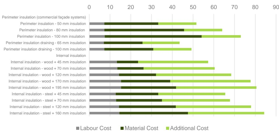
**Figure 6 - Component Cost Sweden – Outer Walls Against Earth (Opaque Components)**
