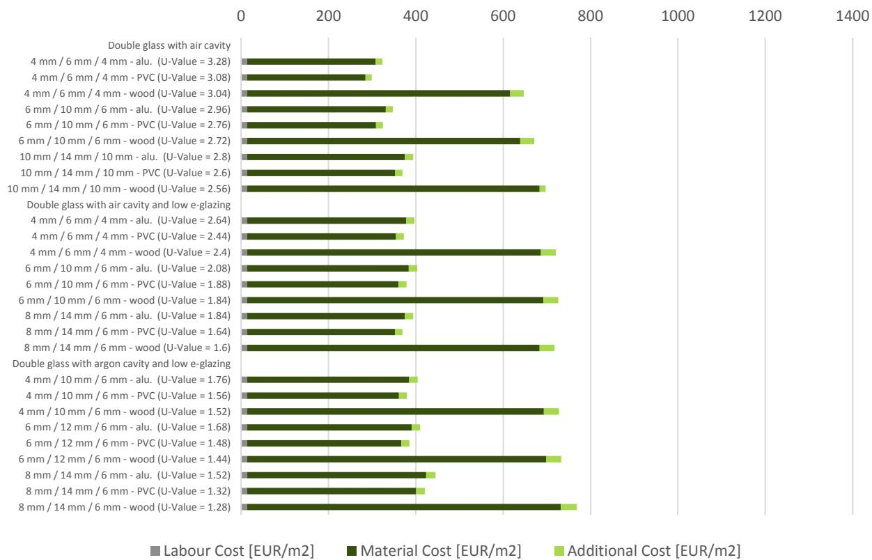
Figure 33 - Component Cost Spain– Windows in tilted roof (windows)
