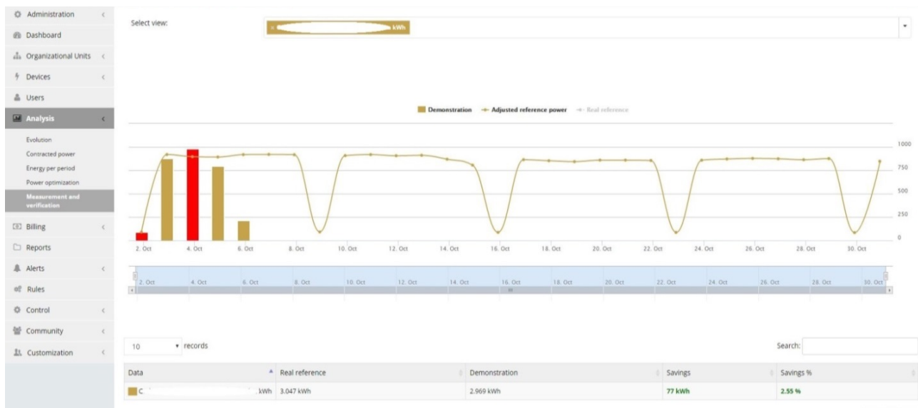
Figure 8: example of an installation’s savings analysis through the calculation of the baseline as function of surface, occupancy and temperature performed by the software.
