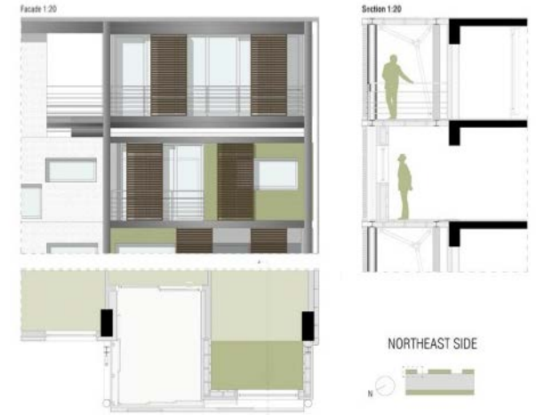
Figure 17. Façade, plan and detailed section of a typical application of the GET system on the Peristeri building.
